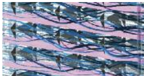
Mixing generated by Delta Wings (CFD simulation)
